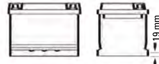
B4 Base holddown 19 mm (on long sides)
